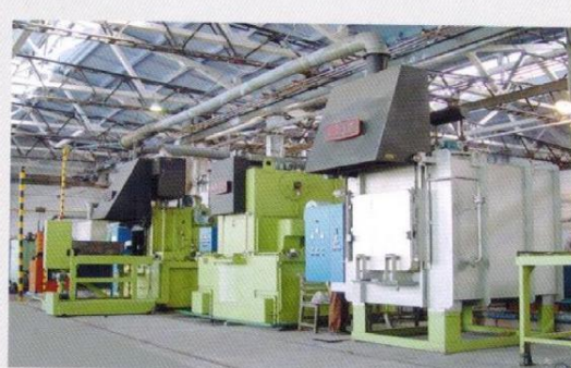
(GCIT) DM21密封多用箱式炉生产线 (GCIT) DM21 Components Manufacturing
